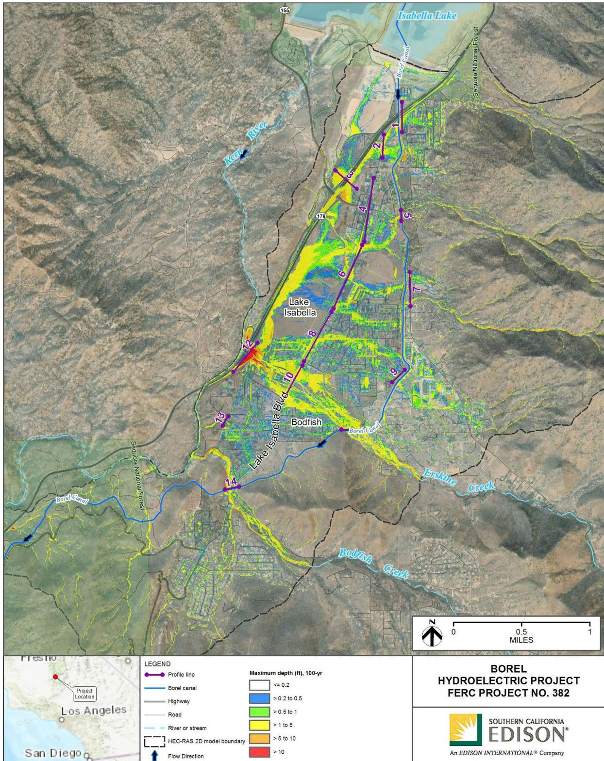
Figure 3-11. Existing Conditions Local Storm Maximum Depth – 100 Year
