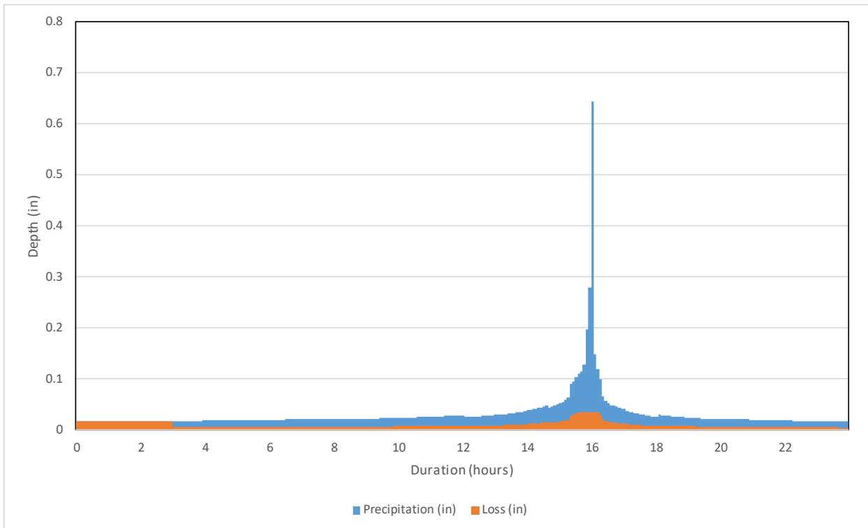
**Figure 3-5. 500-year Precipitation Hyetograph and Loss Time Series**
