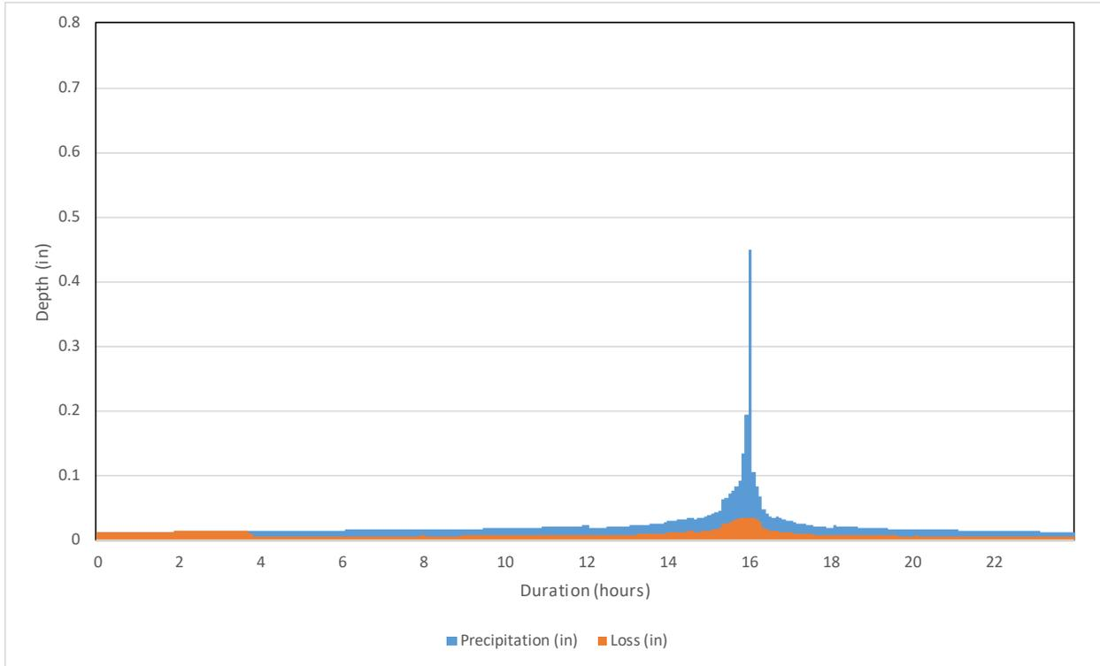
**Figure 3-4. 100-year Precipitation Hyetograph and Loss Time Series**
