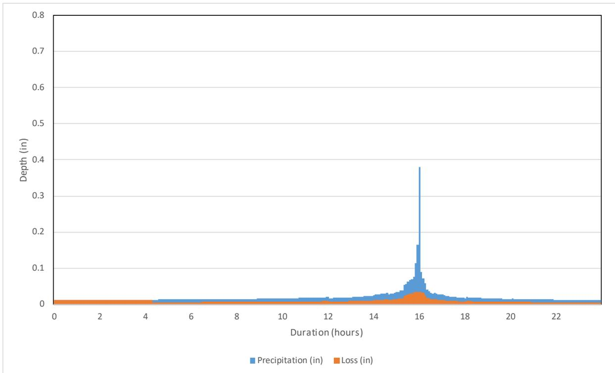
**Figure 3-3. 50-year Precipitation Hyetograph and Loss Time Series**
