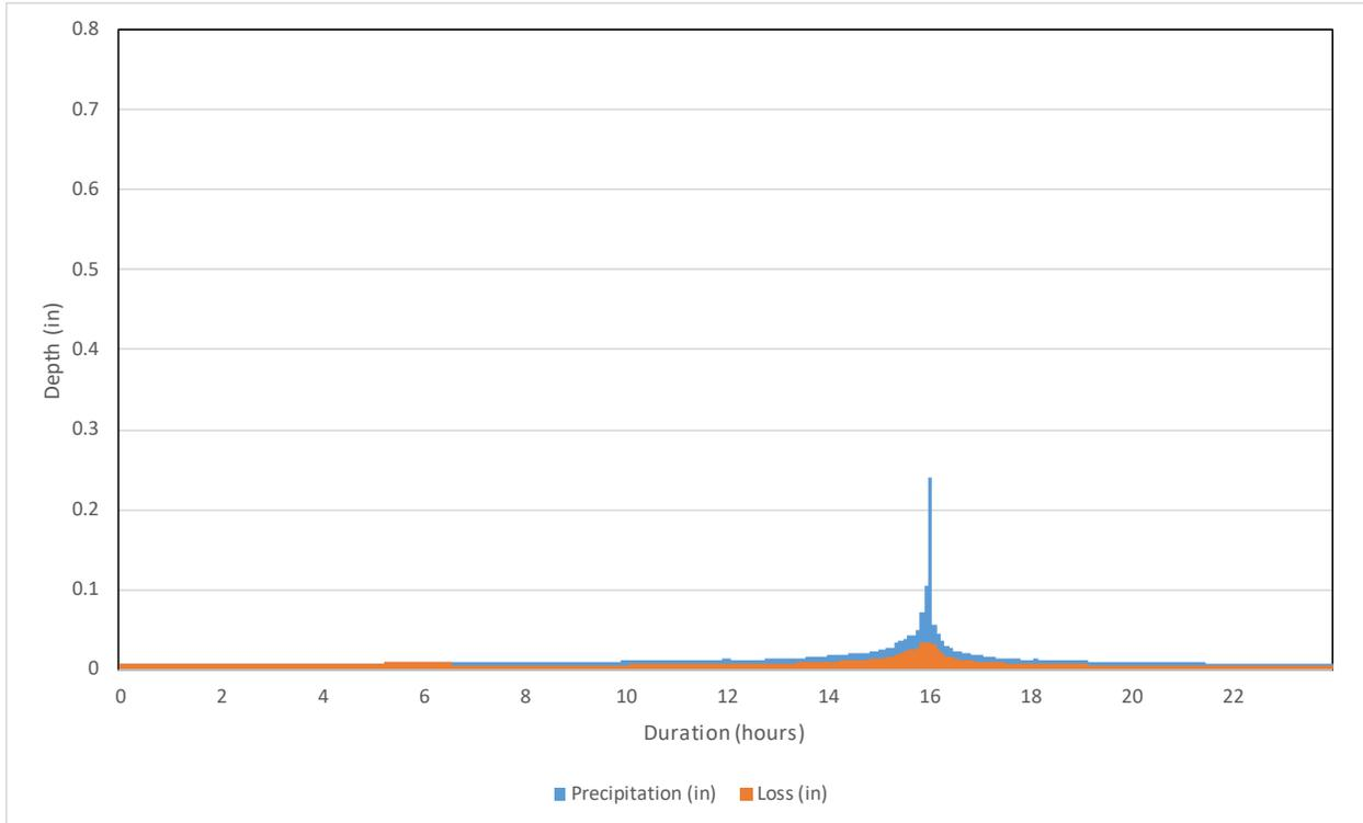
**Figure 3-2. 10-year Precipitation Hyetograph and Loss Time Series**
