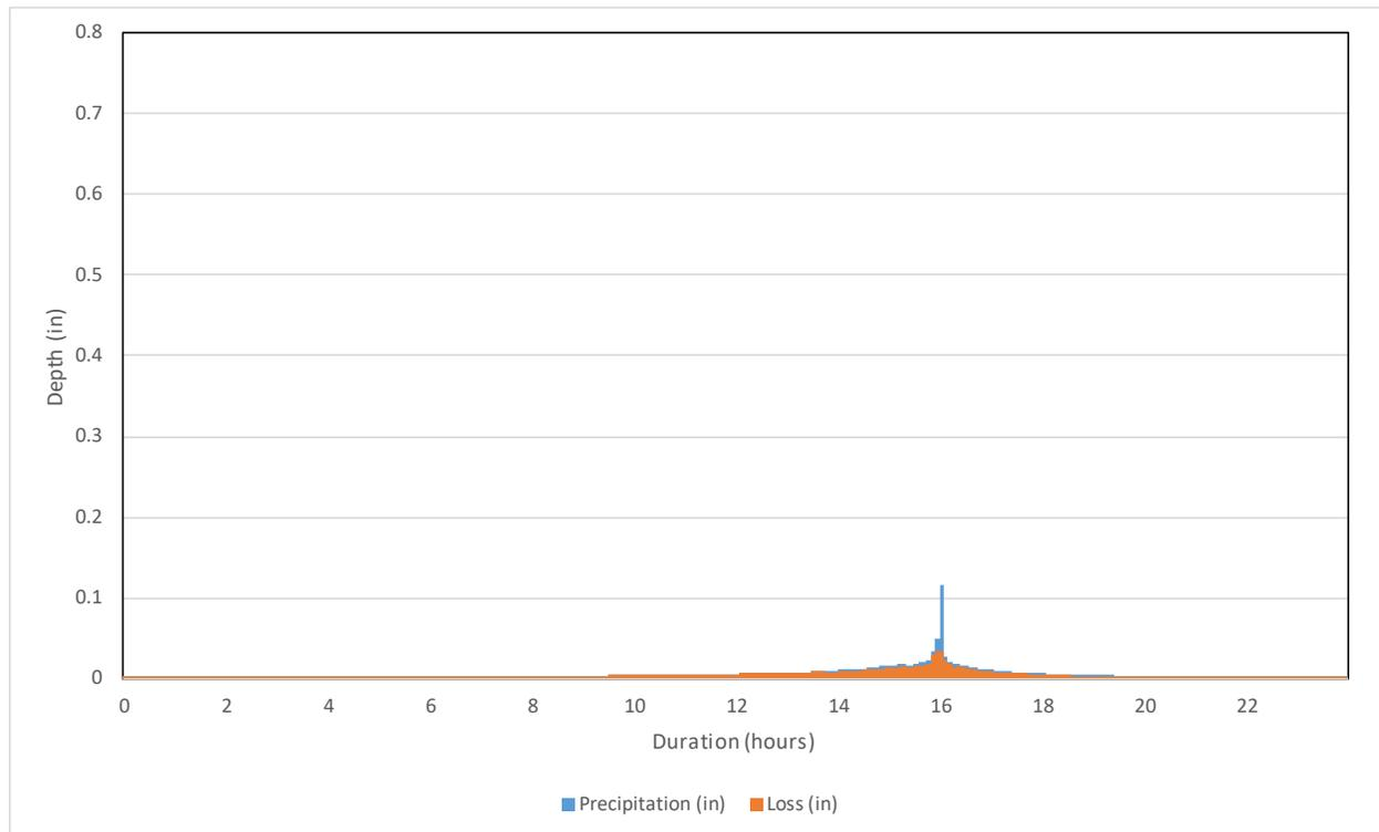
**Figure 3-1. 2-year Precipitation Hyetograph and Loss Time Series**
